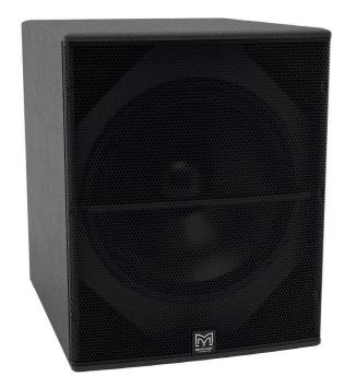
The CSX118 is a compact, high performance subwoofer that extends the low frequency operating range of the combined system to 35Hz and provides exceptional low frequency impact. An ideal partner for the CDD10, CDD12 and CDD15, it features a long-excursion 18" (460mm)/4" (100 mm) voice coil driver with a water-resistant cone and triple roll surround in a compact reflex enclosure.
